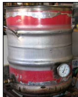
The mash tun sports a full sweep 3 inch Ashcroft 250 degree dial gauge
