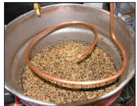
The sparge arm in the mash tun washes the sugars from the covered grains
